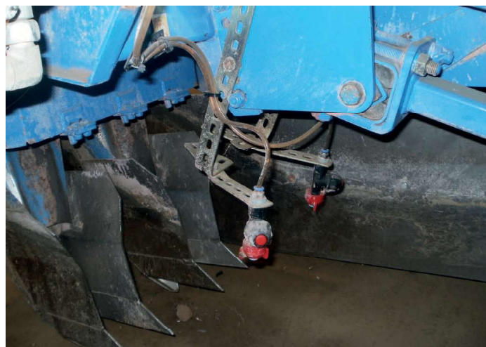
Figure 7. In-furrow application. Top: three-row planter with two nozzles in each shoe. Bottom: quad planter with rear nozzles only
